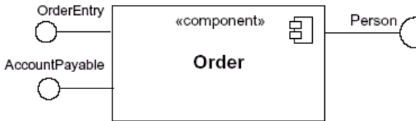
Figure 4: An alternative approach (compare with Figure 3) to showing a component's provided/required interfaces using interface symbols
