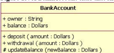
Figure 15: A BankAccount class that shows the visibility of its attributes and operations
