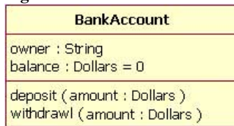
Figure 2: A Bank Account class diagram showing the balance attribute's value defaulted to zero dollars
