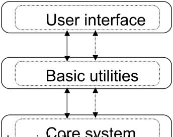
Each successive layer is built on its predecessor, hiding the lower layer and providing some services that the upper layers make use of. Upper layers often form virtual machines.
