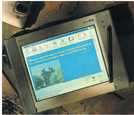
Figure 1. The Guide system consists of a tablet-based PC equipped with IEEE 802.11 wireless networking capabilities.
