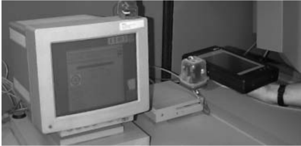
Figure 7: Home-made ir units allow cross-platform communication.
