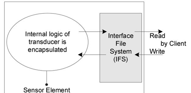
Fig. 12. Interface File System in a Smart Transducer
