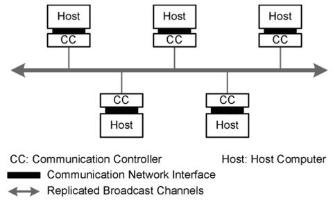
Fig. 2. Distributed Real-Time System with Five Nodes
