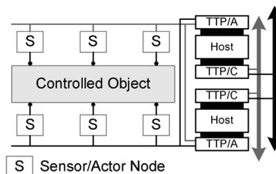
Fig. 13. Replicated Fieldbuses
