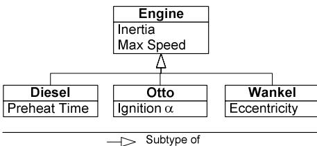
Figure 4. Extended engine class hierarchy
