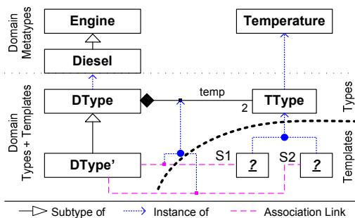
Figure 12. Pre-allocating connector links
