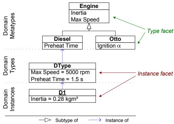
Figure 6. Engine hierarchy with clabjects
