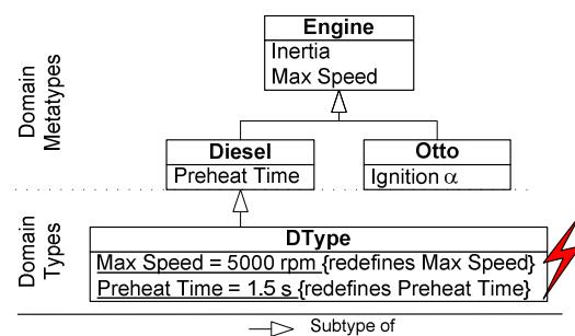
Figure 5. Engine with static attributes
