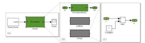
Fig. 3. (a) Simulink model with the TDL module block *Sender*, (b) Generated contents of the Sender module, (c) Sample implementation of the t1Impl task function.
