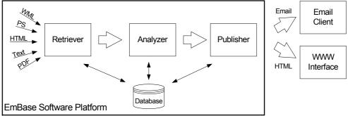
Figure 1. Overview of the EmBase Software Platform.
