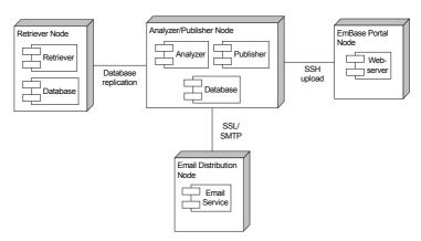
Figure 2. Deployment Diagram. [object Management Group]
