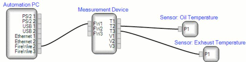
Fig. 1. Sample physical view of a test bed
