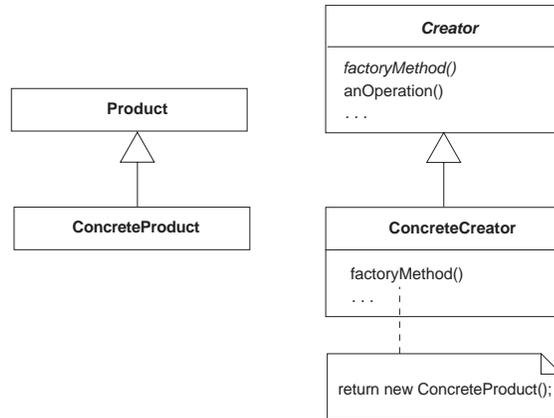
**Fig. 8.** Structure of the Factory Method pattern (adapted from Gamma et al., 1995).
